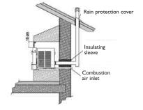
If the stove is installed in a building with potentially inflammable walls, it will be necessary to place an insulating sleeve between the wall and the flue gas exhaust pipe and similarly for the overhanging part of the building's roof.
