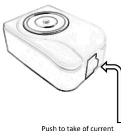
In the absence of the button release, embedded in the electromagnet, press the button provided in the electrical system intended for this purpose. Never force the door to release it from the electromagnet.
