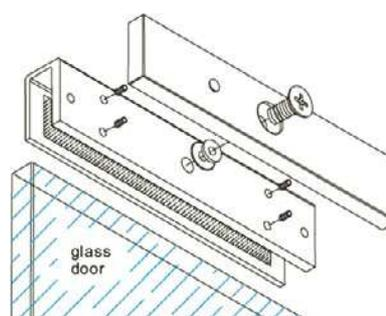
STU BRACKET IS USED TO FIX THE KEEPER PLATE ON GLASS DOOR «TO PUSH», FRAMELESS. IT CAN BE APPLIED IN DIFFERENT THICKNESS GLASSES. THE ELECTROMAGNET FIXING IS TRADITIONAL, IN CASE OF NEED A «L» BRACKET CAN BE ADDED.
